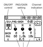
EQ bands are arranged vertically, with matching parameters aligning horizontally. Use the arrow keys to move between the parameters.
