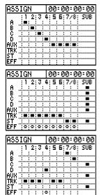
This is the basic RECORDING Quick Setup. Inputs are assigned in order to mixer channels in order. (Input A to Channel 1, Input D to channel 4, etc.) The Aux Input is double assigned to Channels 5-6 and Channels 7-8.
