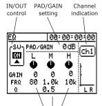
EQ bands are arranged vertically, with matching parameters aligning horizontally. Use the arrow keys to move between the parameters.
