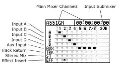
In the above example, you may notice a little circle in the Effect Insert row under Mixer Channel 2. This indicates an effect is inserted into the channel. It could represent the multieffect chain of EFFECT 1, or a channel dynamic from EFFECT 2.
