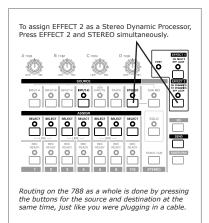
This routing technique means that you don't have to dig through menus to route effects. It's all on the surface of the 788 itself. The specific button pushes for each set-up are shown in the chart above to the right. Refer to it for specific button combinations.
