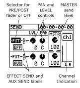
To the right of the LVL and PAN dials is a dial labeled MSTR, which adjusts the overall level of the send. (LVL controls the amount of one particular channel in the send, MSTR affects the level of all the channels.)
